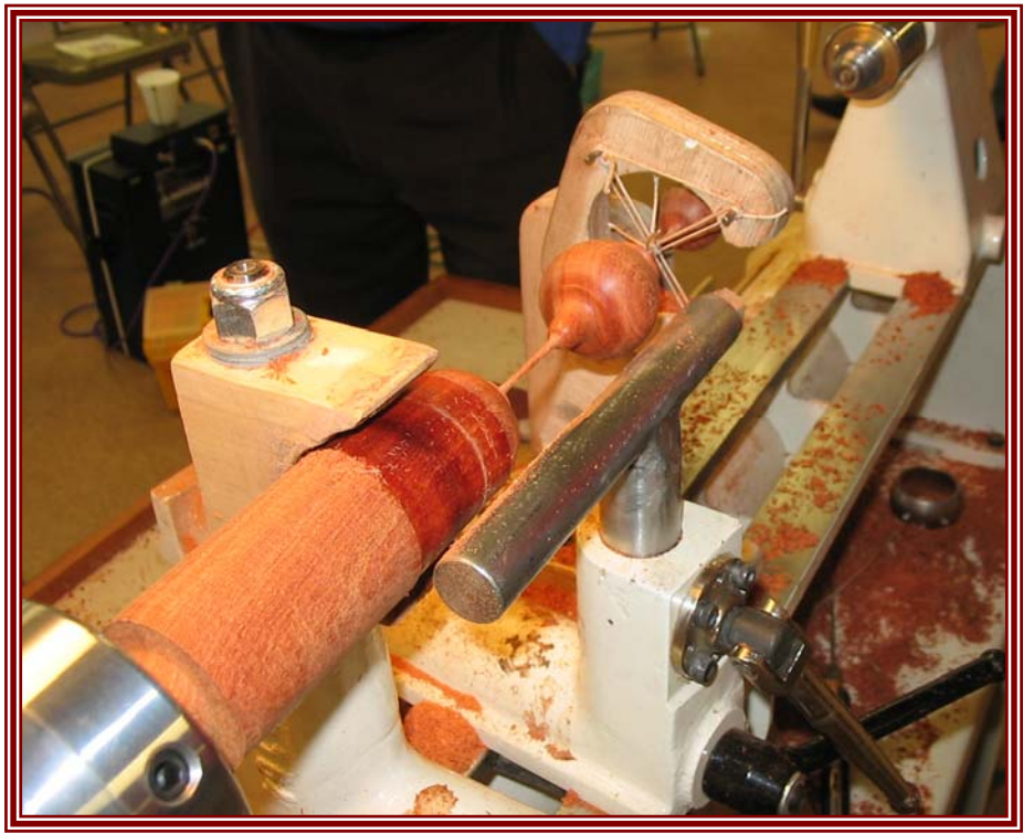
A long turning with a stringed steady rest
