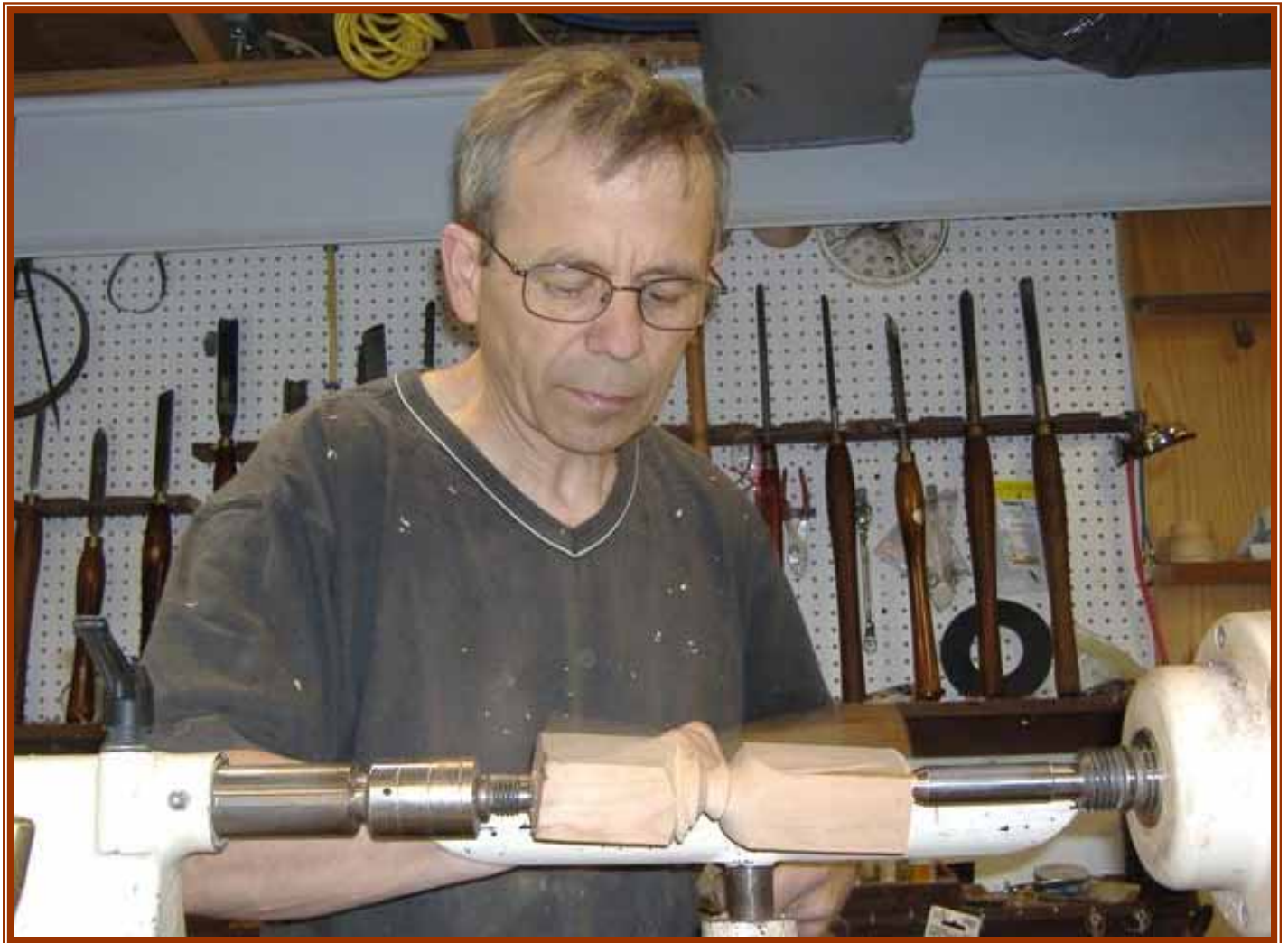
Escoulen turning a piece of Cherry off-center on head and tail ends
