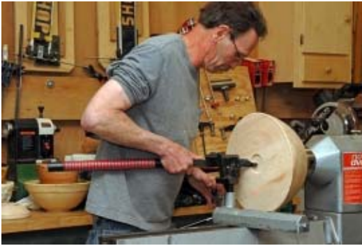
Setting up the corer at the centerline
