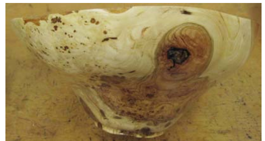
A cherry burl bowl that warped when drying
