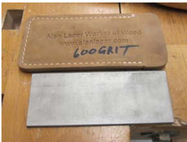
Diamond grit honing stone used for Skews and gouges sold by Alan Lacer
