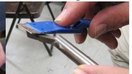
Diamond file putting a burr on hollowing tool
