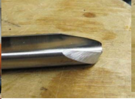
Swept back / fingernail grind bowl gouge
