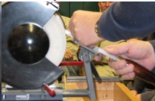
Grinding a scraper using wolverine platform
