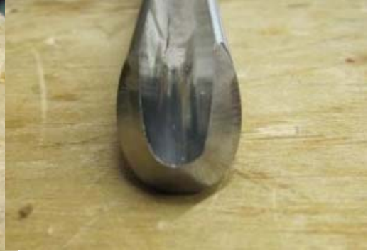
Point view of swept back/fingernail grind bowl gouge
