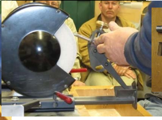
Sharpening using Wolverine jig
