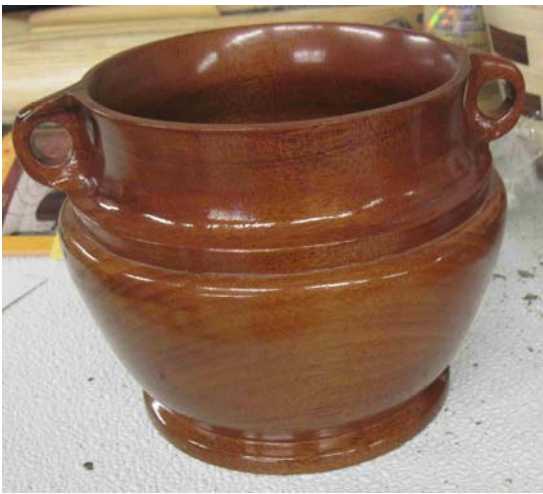
John Chakuroff Mahogany "bean pot" - router was used to cut off section between the "ears" while the unit was mounted on the lathe
