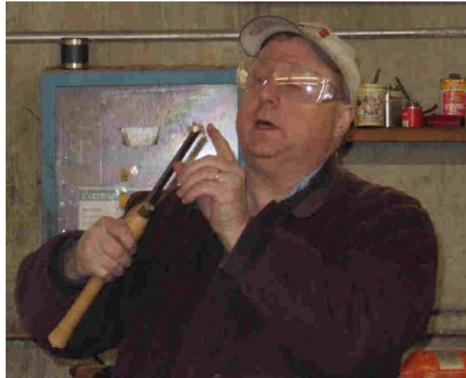
Explaining the bevel and the long swept grind on the 1" wide shallow profile spindle gouge
