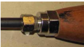
Alternate approach using Compression fitting which can slip if there is a catch
