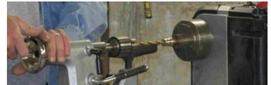
Using Tailstock drill to drill the shaft clearance hole
