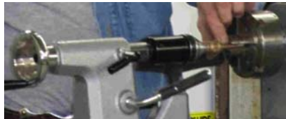
Using the tailstock to center the adapter in the chuck
