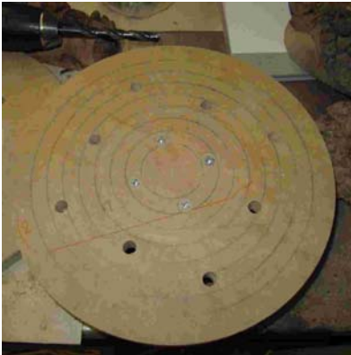
Steel faceplate is fastened to the MDF base.
