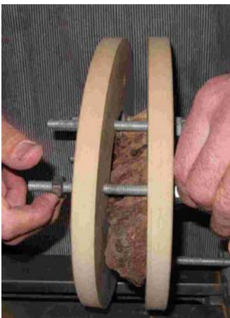
Clamping object inside donut chuck
