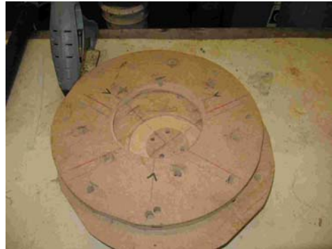
3/4" MDF is used for the donut chuck plates
