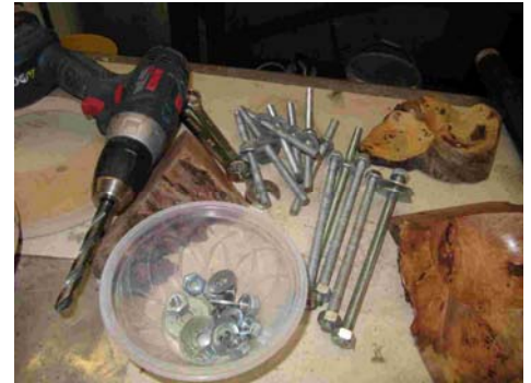
He recommends buying 4 foot lengths of threaded rods and making an assortment of bolts for fastening the donut chuck and offcut together.
