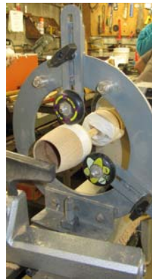
Steady rest stabilizing goblet. The white band at the base of the goblet is tape to prevent the steady rest wheels from burnishing the wood.
