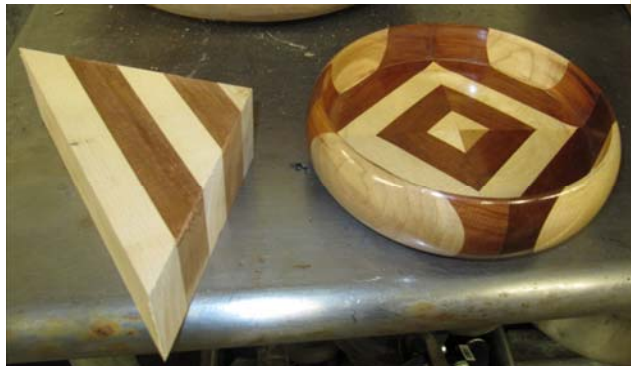
Joe Sheppard showed a "Square" bowl using Maple & Mahogany. "I glued three pieces of Maple & two pieces of Mahogany each about 1" thick. Then cut them at 45°. That gave me the dia. "
