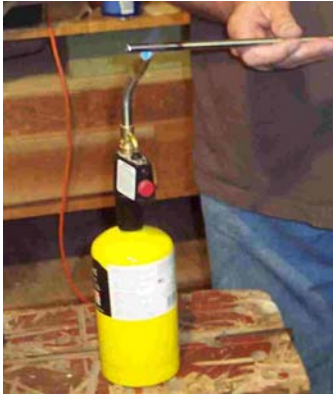
Bending the end by heating the shaft with MAPP gas
