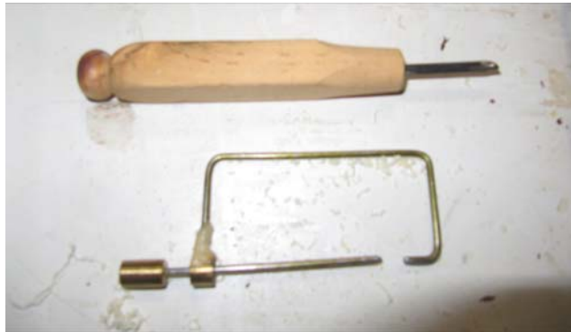
Using a skew as a Negative Rake Scraper to turn an Ivory Palm Nut
