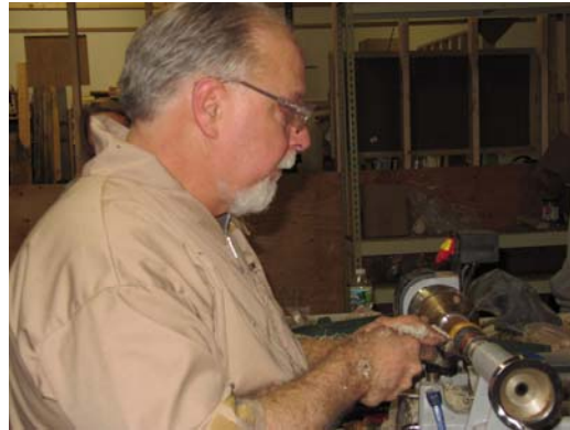
Using a skew as a Negative Rake Scraper to turn an Ivory Palm Nut
