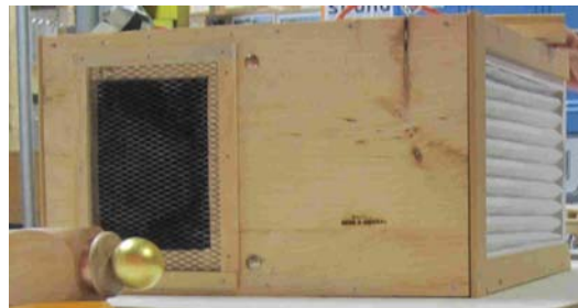
Side view of collector showing exhaust vent
