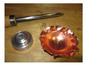
David Hansen showed a tool he made for metal spinning and the first metal items he has tried spinning. The tool had a metal ferrule made from a 1" iron pipe. Copper dish with no support at the end crinkled when he pushed too hard. An Aluminum dish folded on itself. He ended up making an 8" high platform for himself so that he could lean down on the tool while turning. He did buying the OneWay metal spinning tool rest.
