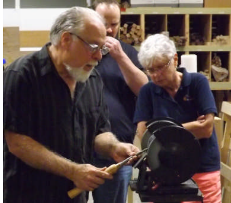
Freehand setting up a long bevel on a gouge while Lorraine Hilton and Garet Holcomb look on
