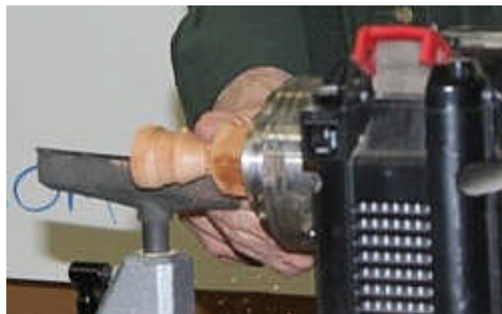
Cutting a tenon on the flower base which will be inserted at the top of the stem.
