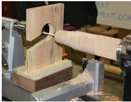
Locating the steady after turning the top portion of the stem.
