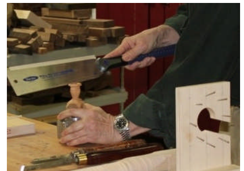
Laying out and cutting the petals on the flower before cutting the tenon at the base.
