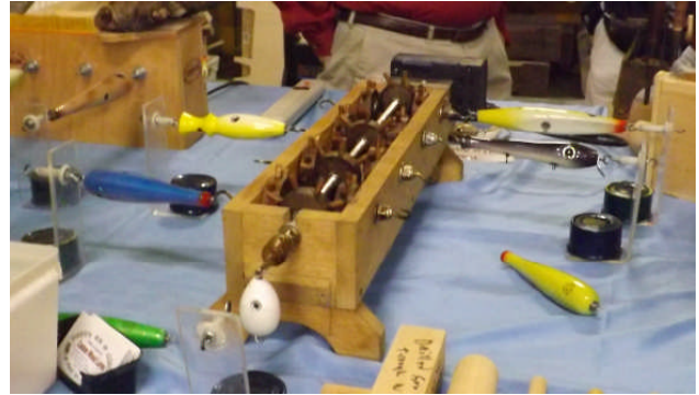
Jig for spinning lures while the Epoxy coating cures
