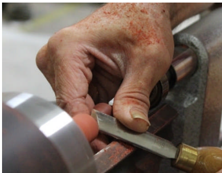
Turning the icicle using a skew and backing up the icicle with fingers
