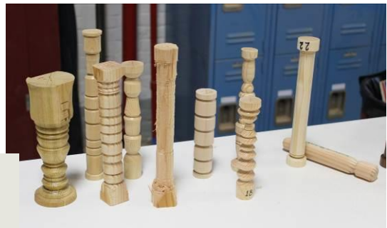
Various spindle-turned pieces, representing a learning process using only a skew chisel
