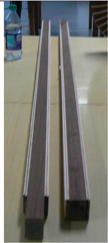
Alex Amoruso The 2 pieces on the right are what is needed to make the platter in the center. They will be cut into 20, 9 inch pieces and then be cut into 40 pieces at 9 degrees.
